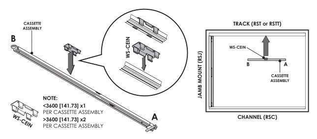
NOTE: Fit WS-CEIN before fitting cassette into the top track (RST or RSTT)
