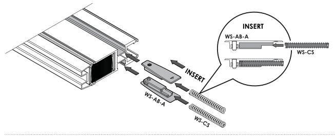
4. Inserting the Friction Block
