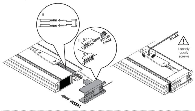
5. Inserting the Mesh Retainer
